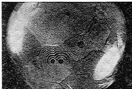
Fig. 1. Typical crystal pattern of methyl mesitylcarbamate from chloroform solution in a 50 cm 3 eggplant type flask.
